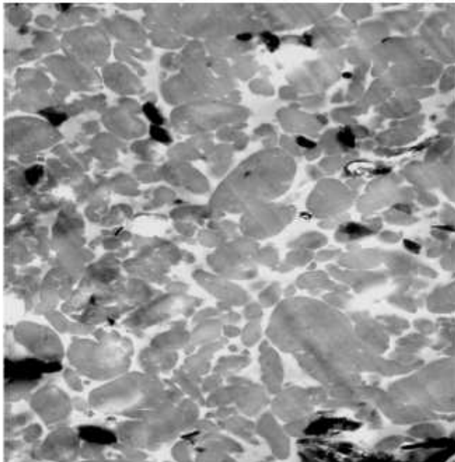
- Transmission electron microscopy (TEM) of PP/EPDM TPV. Dark areas are crosslinked rubber particles.
